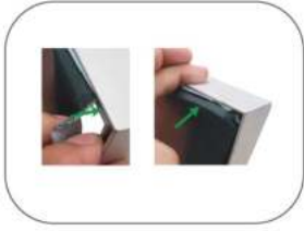
Using your fingers, push both fabric and silicone beading completely into the extrusions channel.
